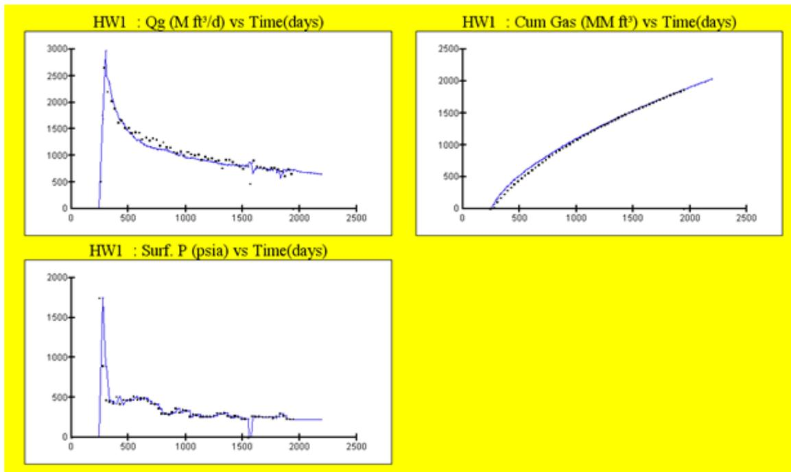
Figure 7 – Match of Well 11 - 240 ft Fracture Half Length
