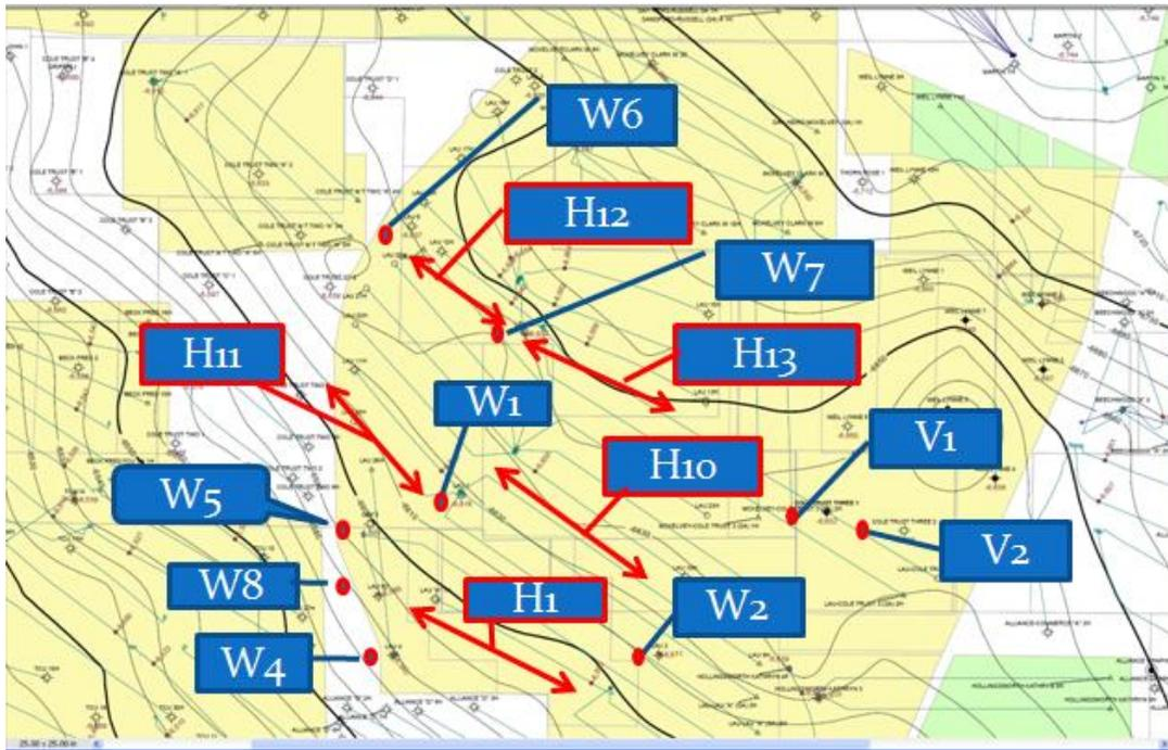
The vertical wells have between 8 and 10 years of historical performance prior to drilling the infill horizontal wells.
