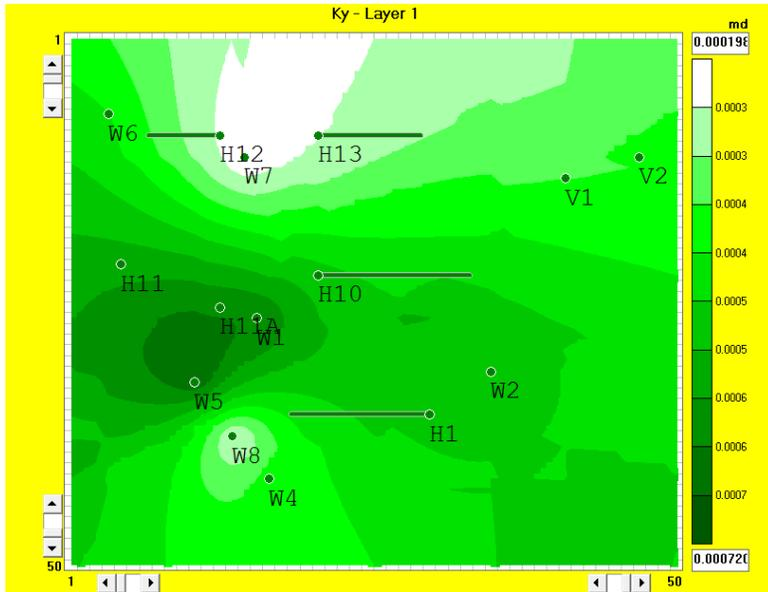
Permeability varied from 200 to almost 700 nanodarcies. The three fold permeability contrast illustrates the permeability variability seen in many tight assets, and the need for accurate permeability maps as optimal economic well spacing is strongly dependent on permeability.
