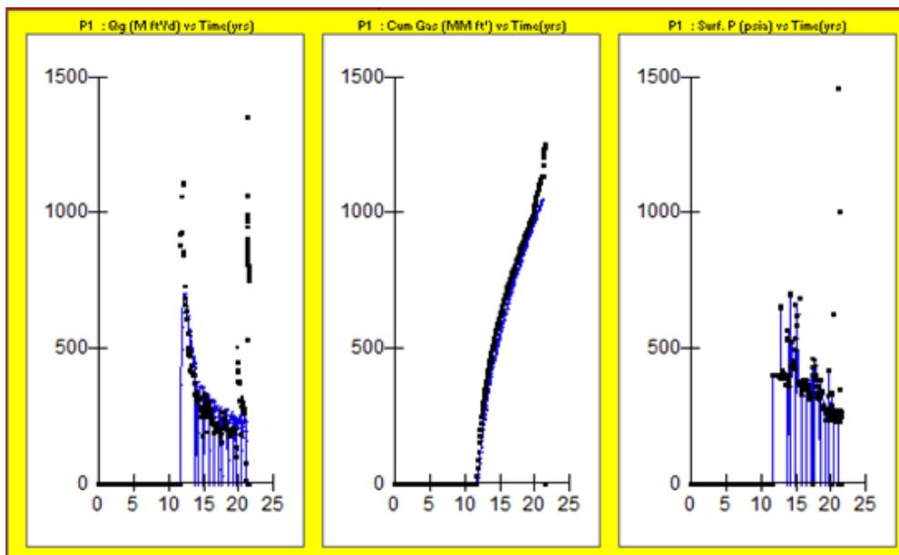
In this instance, the recorded tubing head pressures and historical rates serve to control the well while the assisted history match tool varies the parameters in Table1 (permeability, porosity, and fracture length). Note: The data points around day 8000 reflect a recompletion in the well and were ignored during history matching.
