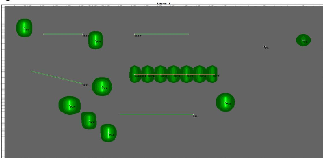
The pressure difference map shows no appreciable inter-well pressure interference. Production and pressure records confirm negligible interference between the vertical or horizontal wells.
