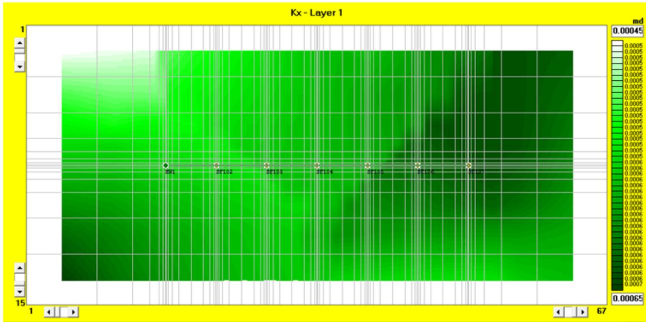
The grid in Figure 5 is refined to 5 feet around the fracture stages and fracture tips to accurately model pressure and saturation changes immediately surrounding the stages.
