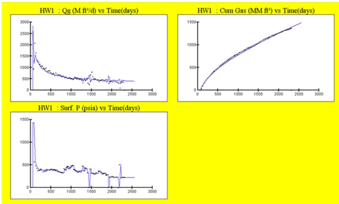
The matches of rates and tubing pressures for all of the horizontal well models are nearly perfect. Indirectly this validates the average permeability map created from the pattern vertical well matches. It is impossible to achieve matches of this quality without having accurate average permeability around each horizontal well.
