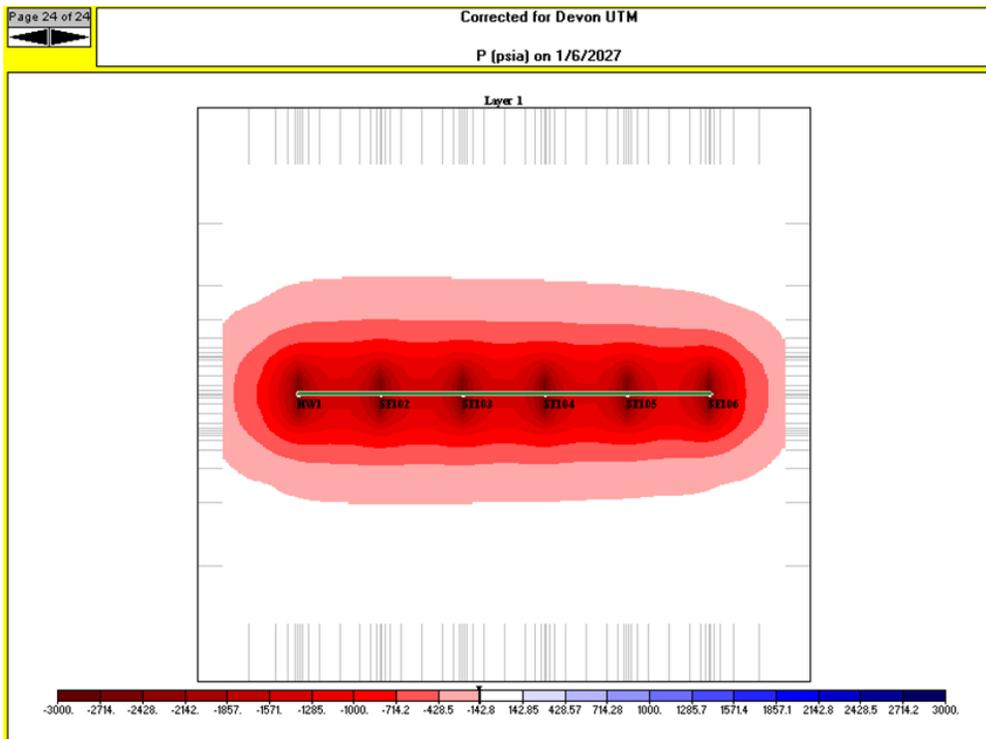
The pressure difference map is not symmetric at each fracture stage because the permeability varies along different parts of the horizontal well.
